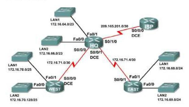
Determine summarized routes that can be used to reduce the size of routing tables
