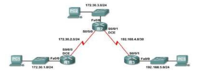
Scenario C: Running RIPv1 on a Stub Network
